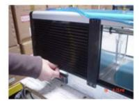
2. Tilt the louver outward a bit and pull it down all the way. Do not force the louver to take it out, but gently shake it side to side a couple times instead and pull it down.
